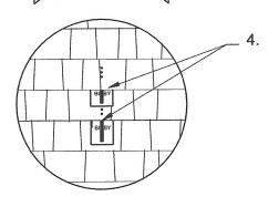
Gently pry up the shingles in these (2) locations and slide the Bibbys underneath the shingles and push down on the shingles until the "Geocel" is oozing out through the holes in the shingle.
