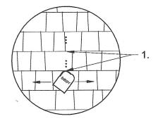
Use serrated edge of BIBBY in a "sawing" manner to cut the "seal" between the shingles in these (2) locations.
