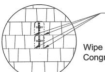
Gently tap the "tab" locations with a hammer (imbedding the tabs partly into the shingle below).
