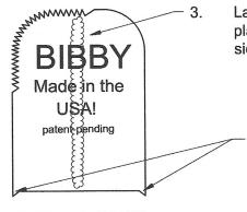
Lay a thin line of Geocel here and place a single "dab" on the back side.
