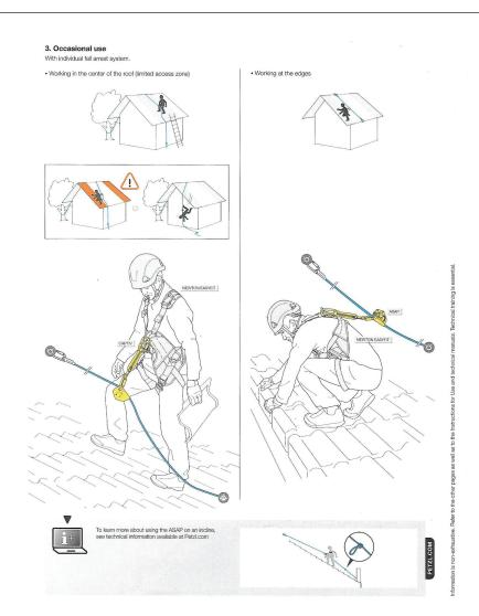
Installed on a safety rope, the ASAP and ASAP LOCK mobile fall arresters connect to the harness sternal or dorsal attachment point. They follow the user in his or her movements, and, in case of a shock load or sudden acceleration, they lock and stop the fall.
