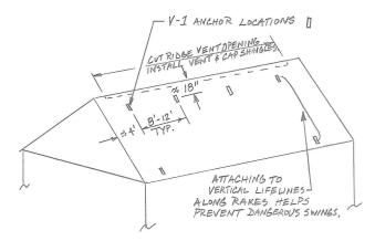
Although it is preferable to have the anchor point in the line of sight, the V-1 anchor system may be used to work over the ridge at certain times.
